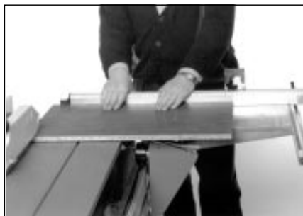
Swing flipstop up and place workpiece on table. Start saw and square workpiece.
